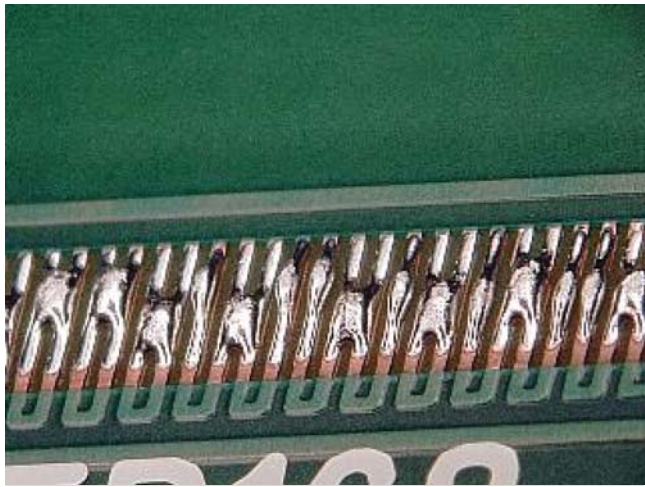
Figure 1-6 Bridging or Poorly Defined Solder Paste Printing
